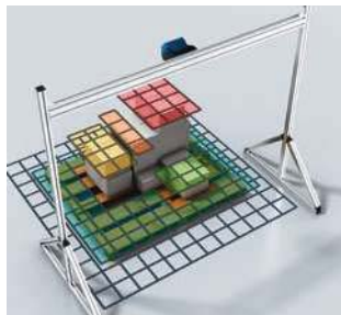
Cartesian data reduction: Selection of the required measurement volume and output of data in Cartesian coordinates (X-Y-Z).
