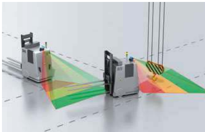
Detection of objects on and above ground, such as the manned forklift trucks or cranes shown here.
