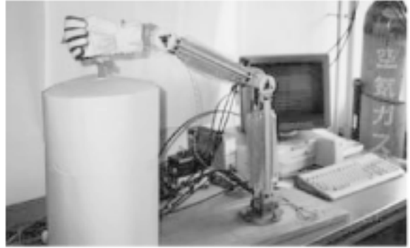
FIGURE 52: PROXIMITY SENSORS ALLOW A ROBOTIC ARM TO SAFELY HANDLE FRAGILE COMPONENTS
