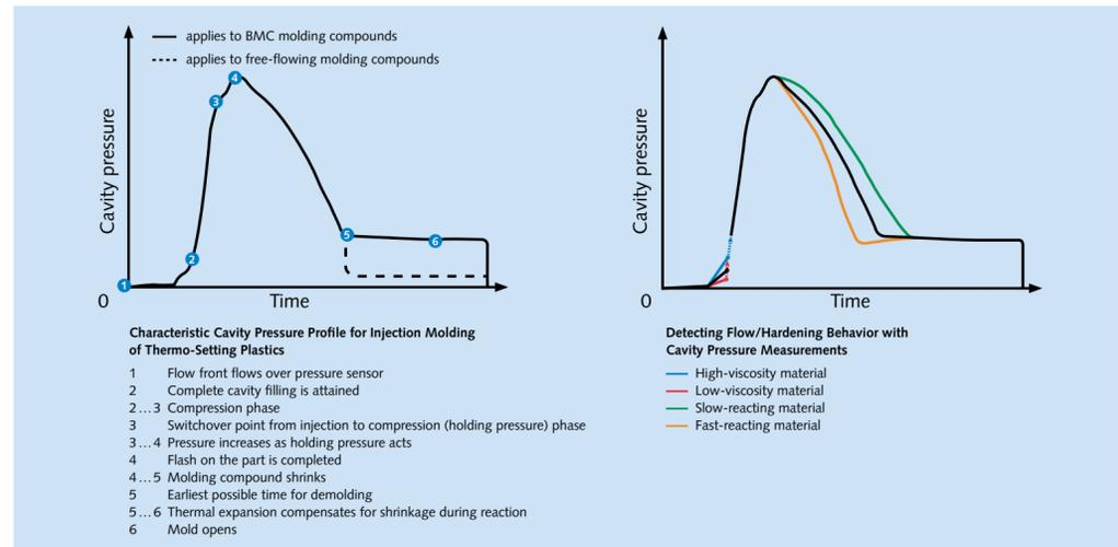
The cavity pressure profile provides information about the quality of each individual part. Knowledge of the fundamental physical relationships makes it easy to evaluate and interpret the pressure profile. The results are guaranteed: sustained quality improvement and reduced scrap.
