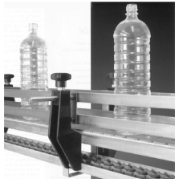
FIGURE 67: A CAPACITIVE PROXIMITY SENSOR "SEES THROUGH" A WALL TO FIND THE TARGET
