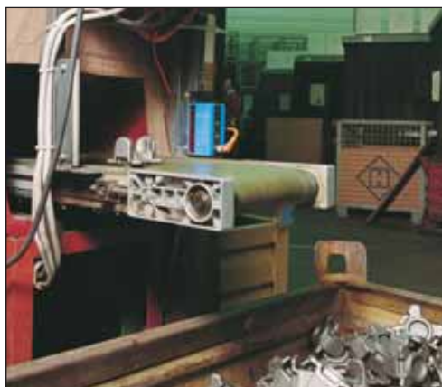
Fig. 4 Counts irregularly shaped objects during production
