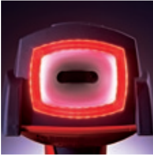
All LEDs engaged, for full light applications e.g. with low contrast codes
