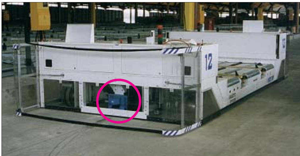
Fig. 5: Collision prevention on an AGV (air freight).
