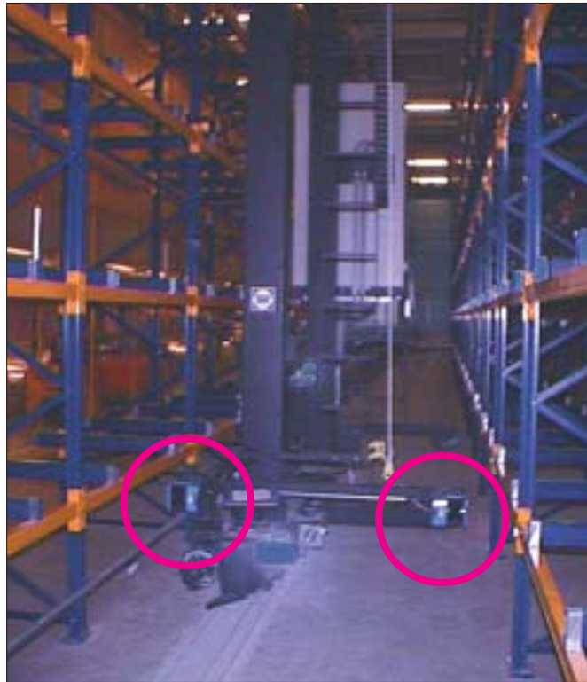
Fig. 6: Checking overhang in a high-bay warehouse.
