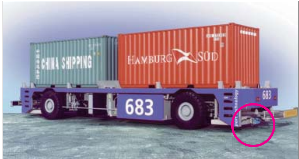
Fig. 4: Collision prevention on an AGV (container).
